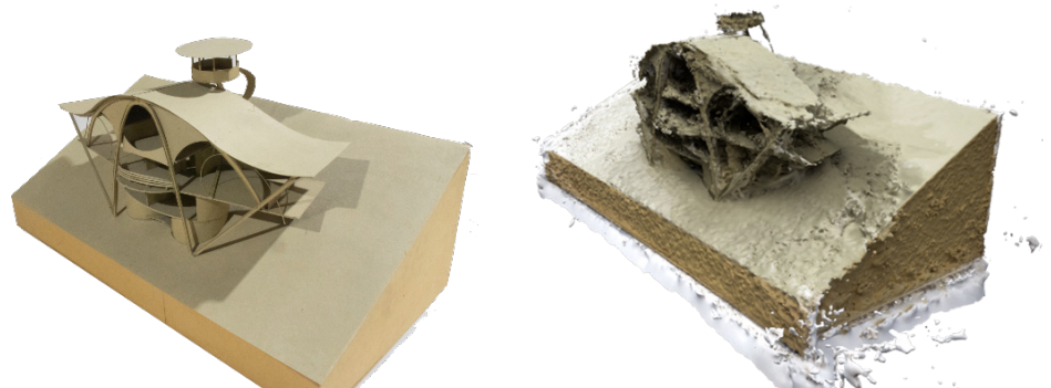
Fig.5. Comparison of model photograph used for photogrammetry (left) and resulting digital model (right). Note the inability of the software to recreate orthogonal members, or flat, single surfaces.
