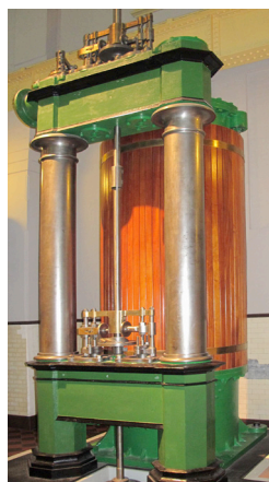
Figure 2. Steam Engine Cylinder with Fairbairn drop Valves, 1856. Museum of Applied Arts and Sciences.
