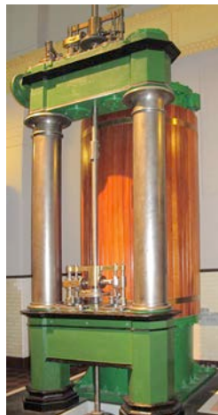
Figure 2. Steam Engine Cylinder with Fairbairn drop Valves, 1856. Museum of Applied Arts and Sciences.
