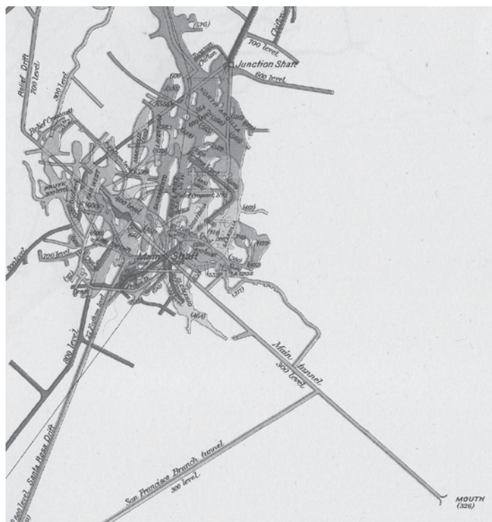
Figure 4. Plan of Early Mine Workings (1840s and 1850s). Early mine workings were created by El Sistema del Rato, or the system of the moment. In this mining method, used by Mexican miners at New Almaden, miners followed ore wherever it led, removing only that rock necessary to follow the ore. (Plan compiled by F. Reade to accompany Becker, Geology of the Quicksilver Deposits of the Pacific Slope [Washington: Government Printing Office, 1888])
