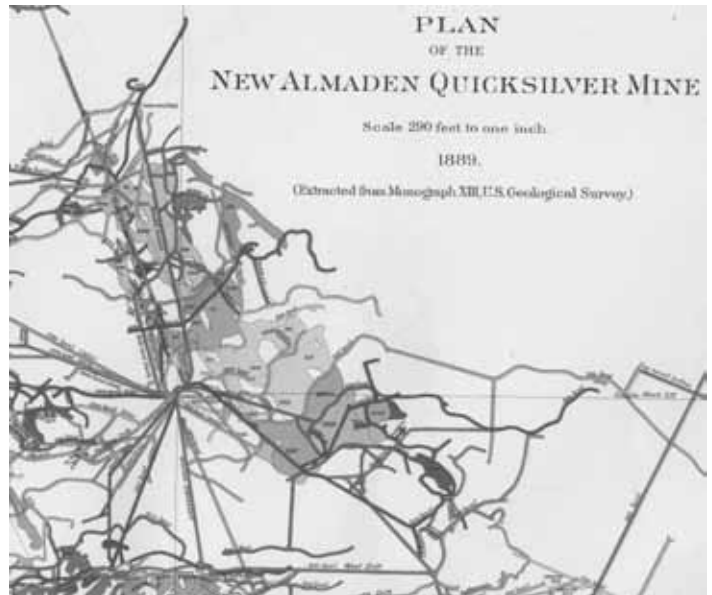
Figure 5. Plan of the Underground Workings at the New Almaden Mine, early 1880s. This plan of the underground workings at New Almaden shows the physical, built legacy of the various mining methods used in the construction of the mine. (Plan compiled by F. Reade to accompany Becker, Geology of the Quicksilver Deposits of the Pacific Slope [Washington: Government Printing Office, 1888])
