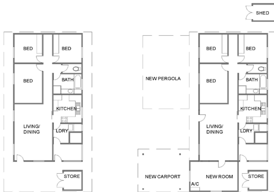
FIGURE 4 a 3-Bedroom Standard Nabalco House at left and an indication of the successive improvements at right including a new room, pergola, carport and shed. Source: LJ Hooker & RTA, Nhulunbuy, 2015.
