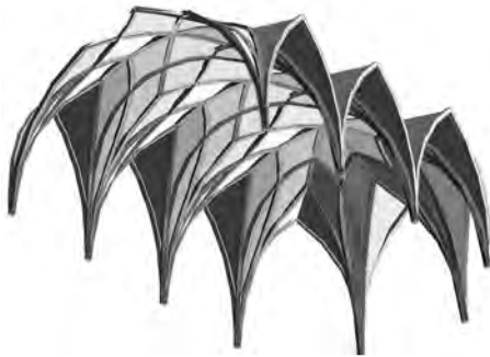
Fig. 6. Rendering of the underside of the chapel vault depicted in the composite drawing fol. 235 of the Stromersches Baumeisterbuch 1 (fig. 3). Drawing by Ross Anderson.
