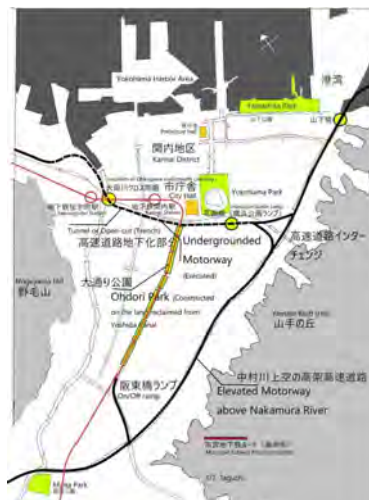
Figure 15. The finally agreed part of underground motorway (dotted line) and its connecting elevated motorways above Nakamura river (Drawing by Toshio Taguchi).
